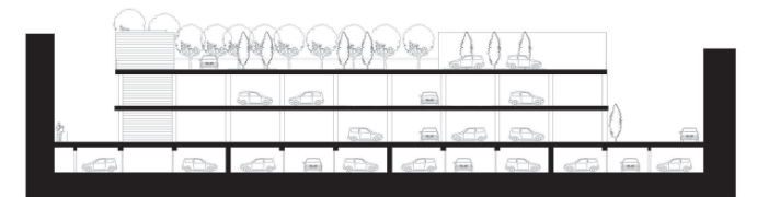
The project: top, the plan for the panoramic area placed on the cover, with the greenery, equipped seating areas and services. The car park is conceived as a hanging garden structure. Bottom, the schematic cross-section of the multi-storey car park.
